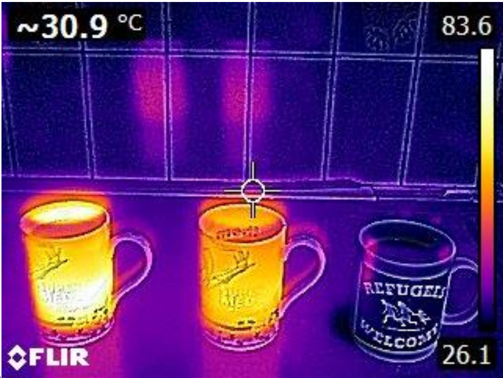
Fig. 7: Cups immediately after filling the two outer cups and emptying the middle cup. Empty cup
